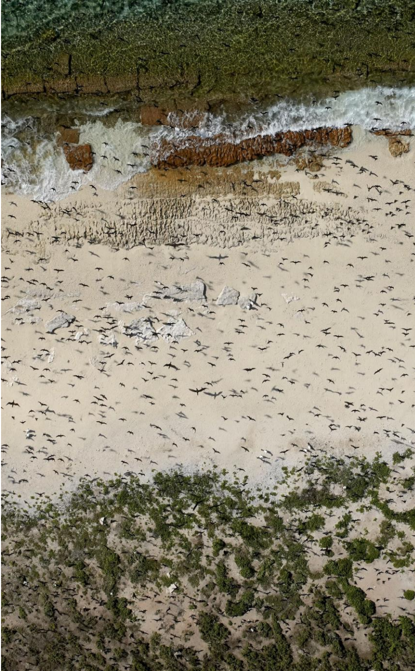
Figure 10-5 birds flying over the sand cause issues with generation of tie points in SfM processing
