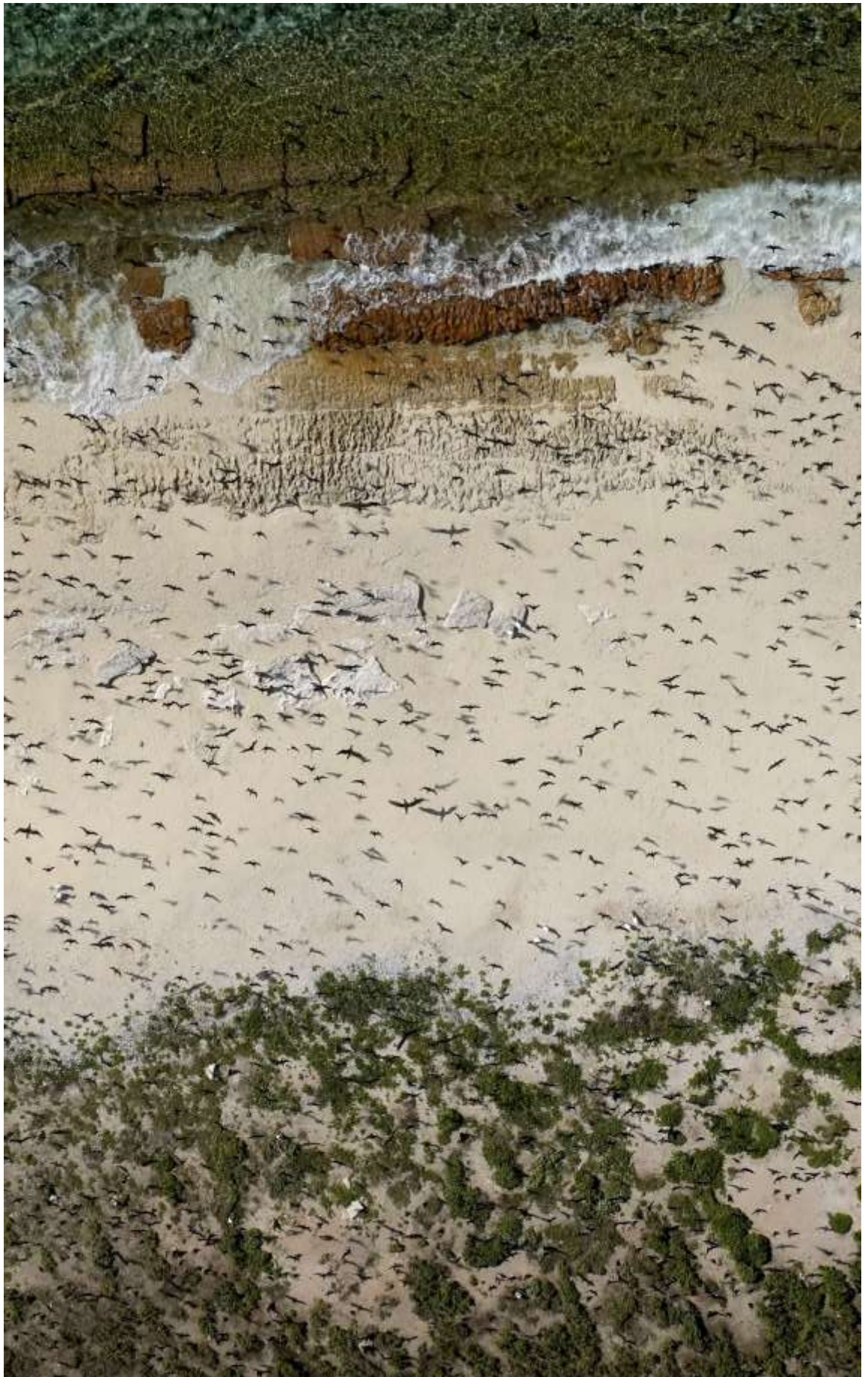
Figure 10-5 birds flying over the sand cause issues with generation of tie points in SfM processing
