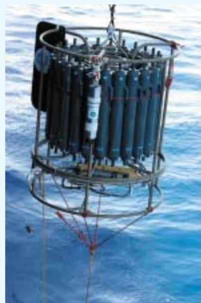
A conductivity, temperature and depth sampler
